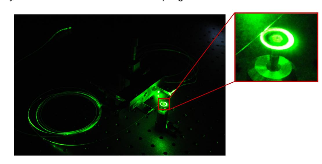
Optical-frequency comb generators can be made of a wide variety of WGM resonators. In this study, we focus without loss of generality on spherical MgF2 resonators with free spectral range (FSR) of about 10 GHz and a pumping wavelength of 1560 nm.
